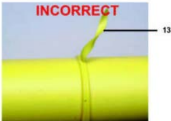
13. Incomplete face off or failure to remove faced off ribbons
