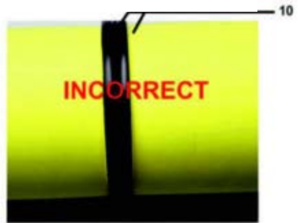
10. Excessive heat time or pressure applied during heating; melt bead too large
