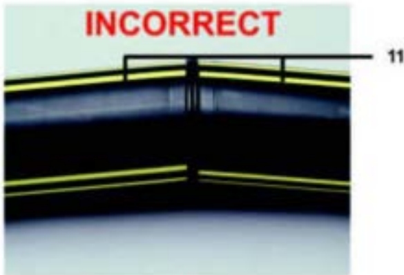
11. Pipe angled into fusion unit
