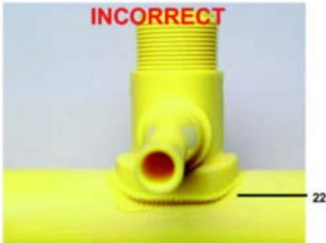
22. Insufficient melt and misaligned
