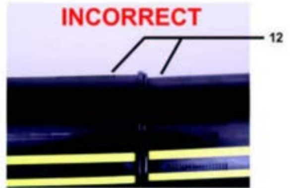
12. Improper "High-Low" alignment
