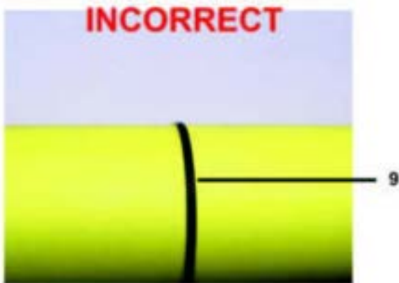
9. Insufficient heat time; melt bead too small
