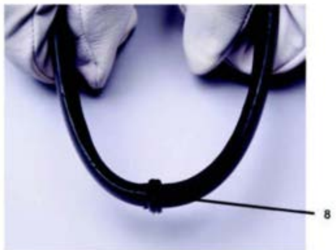
8. No gaps or voids when bent
